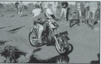
Bad luck for Jeff Leisk, and yet more proof that it's not easy to beat the desert. Running in 2nd spot on the way back, his chain guide wore the ends of the connecting link down so that the clip flicked off and the master link broke – a problem caused by the smaller rear sprocket. He repaired it to finish 82nd outright.
